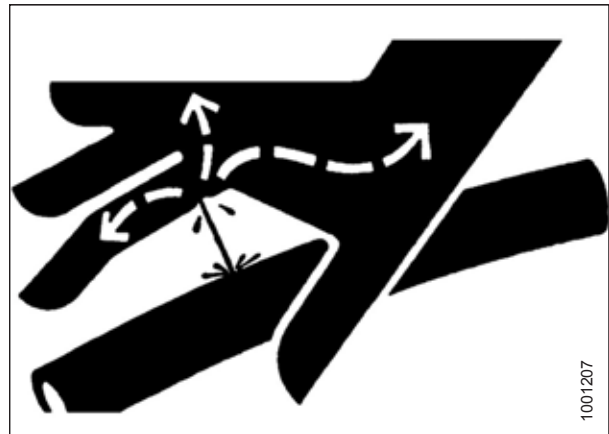
Figure 1.12: Hydraulic Pressure Hazard
